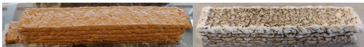
Figure 5. A freshly printed (left) and cured (right) test beam.
