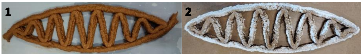
Figure 13. The freshly printed (1) and cured (2) beam.
