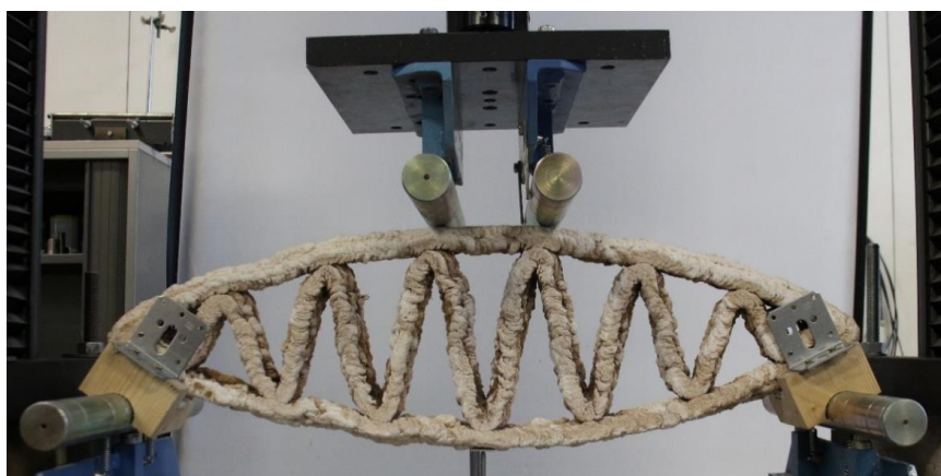
Figure 16. Structural beam test setup up.
