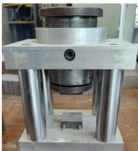
Figure 7. The rigid steel frame of the compression test setup.
