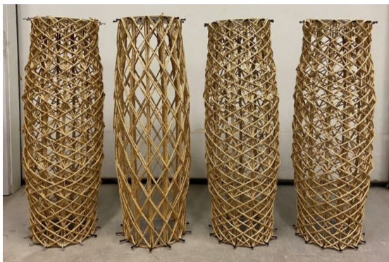
Figure 6: Filament Winded Column [22]
