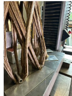
Figure 58: Delamination of bundles
