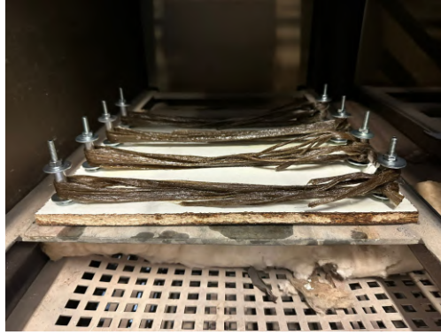
Figure 40: Uncured bundle of fibers of first impregnation test
