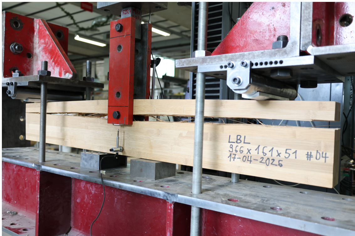
Figure 3.18: Representative fractured splitting specimen, edgewise 966 x 161 x 51 mm TL geometry.
