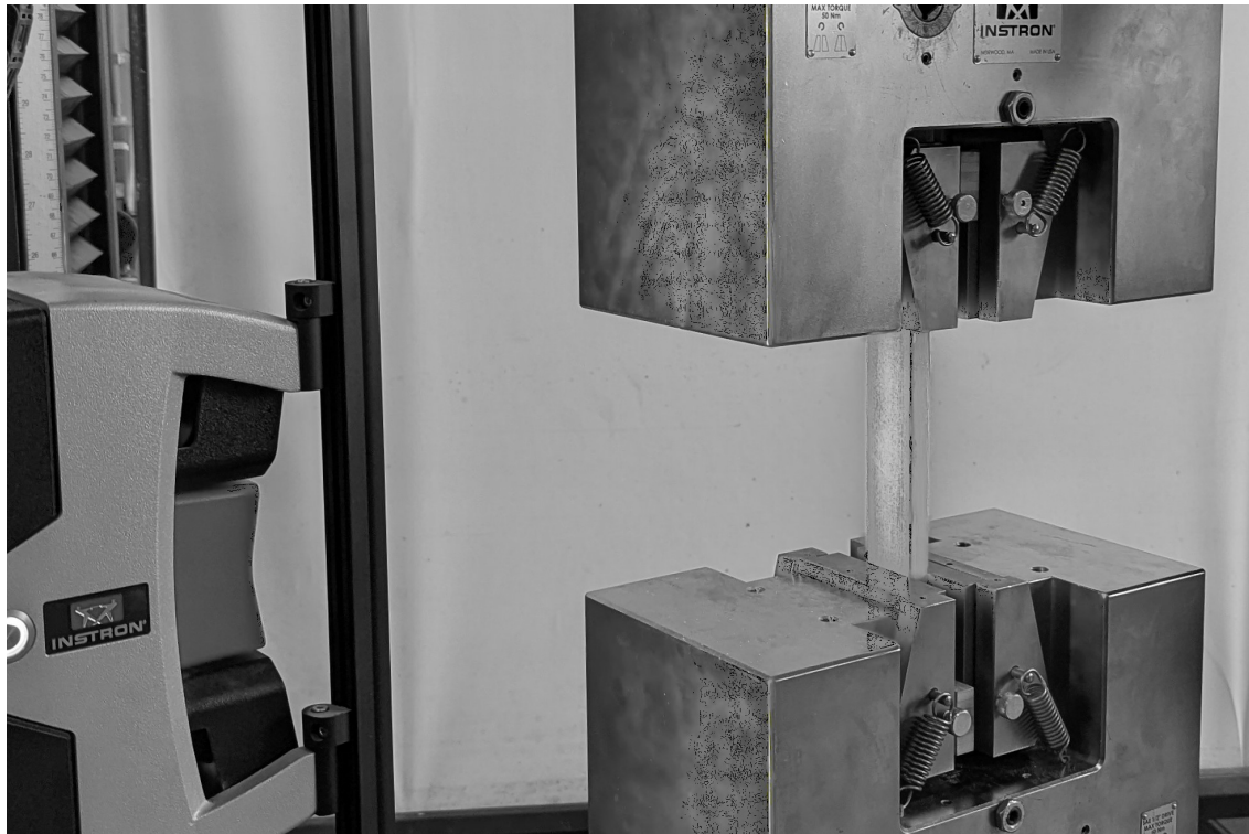
Figure 3.13: Tensile test setup. Rectangular LBL specimen clamped between Instron grips for the parallel-to-grain (TT-L) test.
