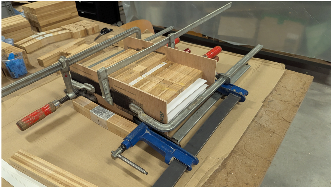
Figure A.1: SENB specimen preparation. Bamboo lamellae clamped during glue cure to form the three-element specimen with the central cube rotated to the target crack system.
