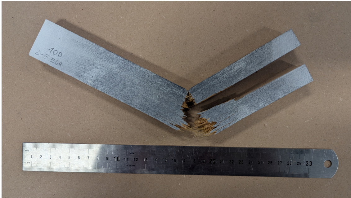
Figure A.22: Fractured ENF specimen after Mode II testing, mid-span V-failure shown with ruler for scale.
