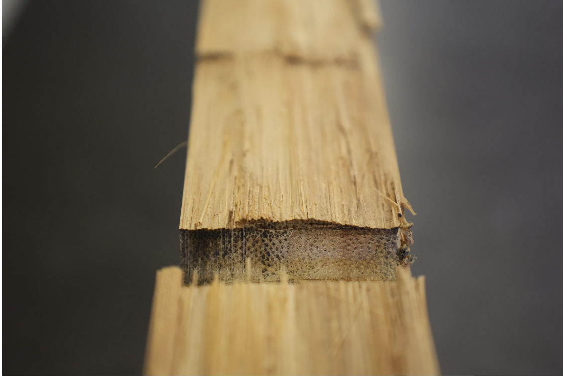
Figure 3.19: Detail view of the fracture surface at the dowel hole.
