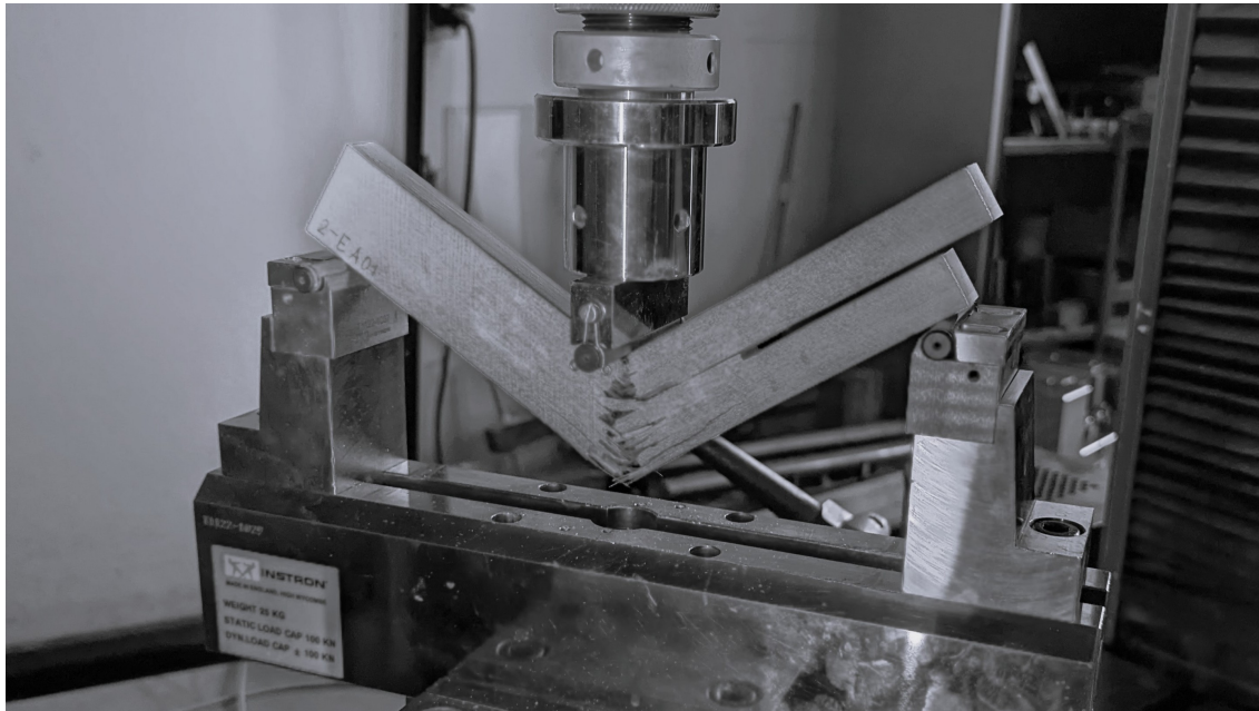
Figure 3.12: Representative fractured ENF specimen after a Mode II test.
