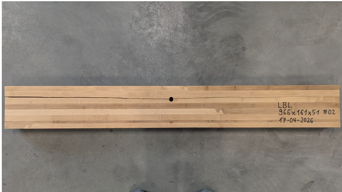
Figure A.40: Fractured splitting specimen (LBL 960 \times 161 \times 51 mm TL) showing the dowel hole and the horizontal split running along the grain.
