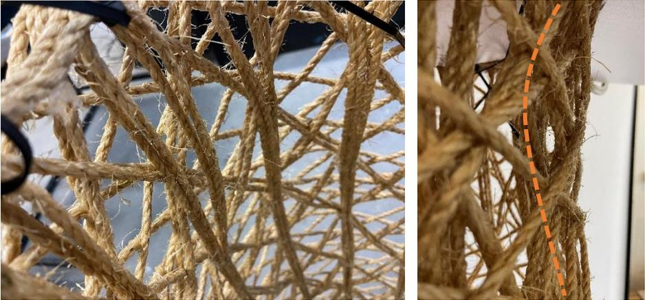
Figure 73 Visible local buckling of the sisal rope after testing
