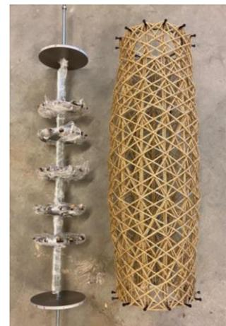
Figure 53 Removed internal formwork after curing →
