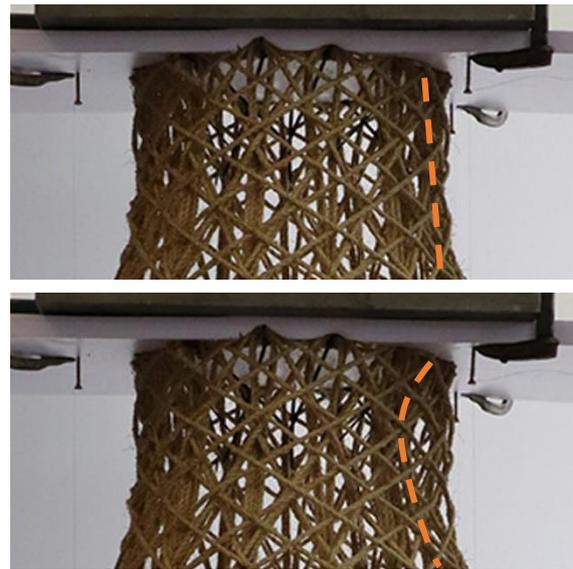
Figure 70 Local buckling occurring during axial compression test column 4
